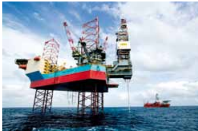
Mærsk Innovator drilling a subsea well using a marine riser
