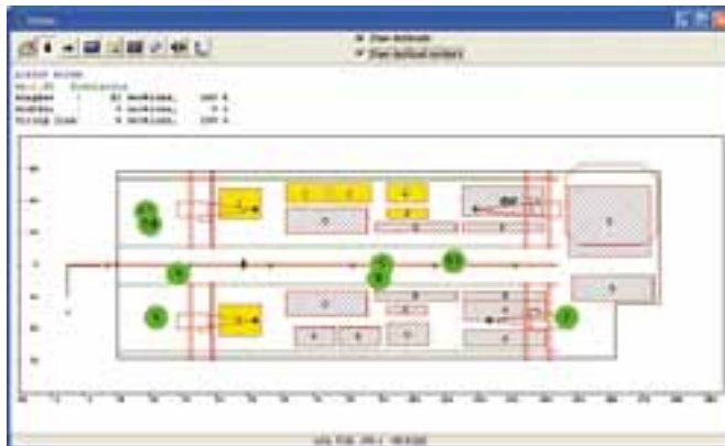
Schematic topview of Acergy Piper (now Castoro 7) pipe laying barge showing pipe storage areas and firing line
