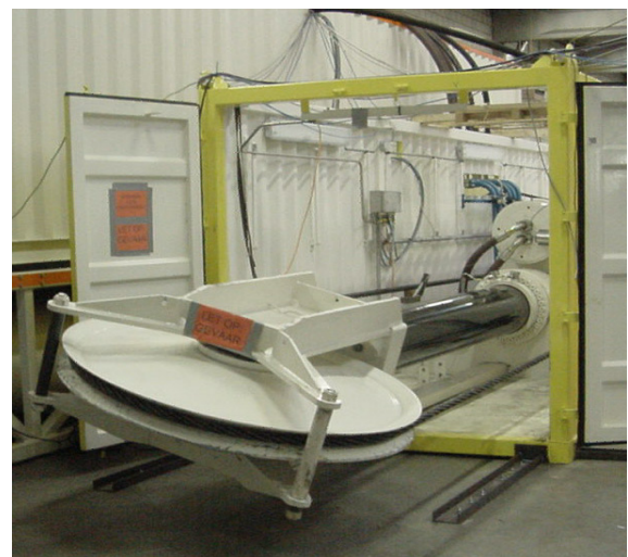
AHC 175 / 40 / 6200 during tests under full dynamic load
